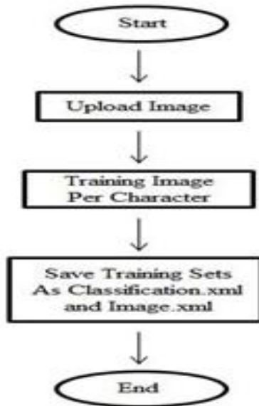
Figure.19: Program Flowchart of training images in La Fila Converter
